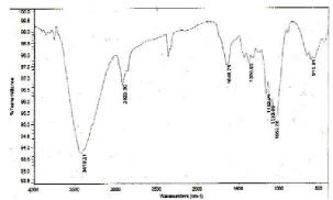
Fig. 6: FTIR spectrum of silver nanoparticles synthesized using mango peel broth.
