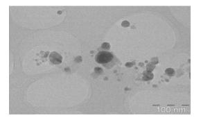
Fig. 4: TEM image of silver nanoparticles
