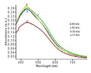
Fig. 1: UV-Vis spectra of silver nanoparticle
